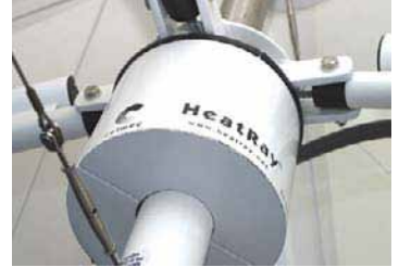
Wiring loom access cover
